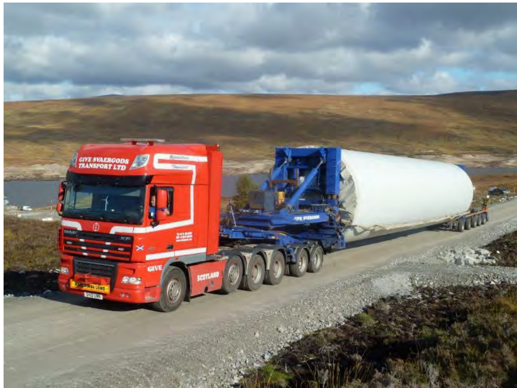
Photo 2.2: Indicative Rear Clamp (Clamp & Clamp) Delivery Vehicle
