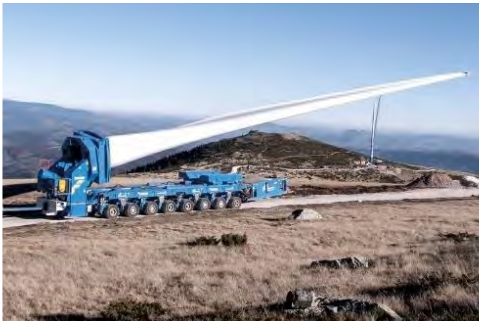
Photo 2.4: Scheuerle Blade Adaptor Delivery Vehicle
