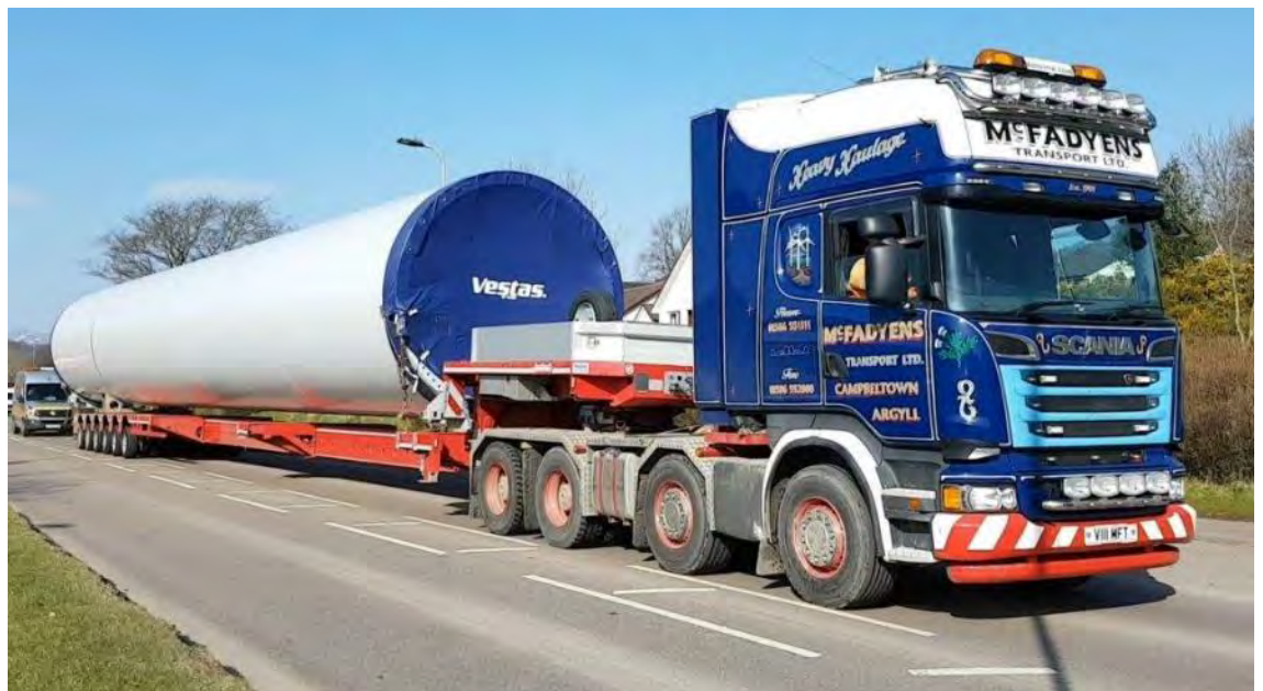
Photo 2.3: Indicative Step Frame Trailer Delivery Vehicle
