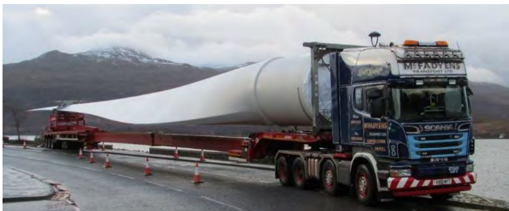
Photo 2.1: Indicative Super-wing Carrier Trailer Delivery Vehicle
