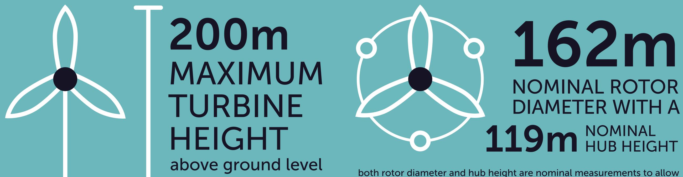
both rotor diameter and hub height are nominal measurements to allow for a competitive tender process across multiple turbine manufacturers
